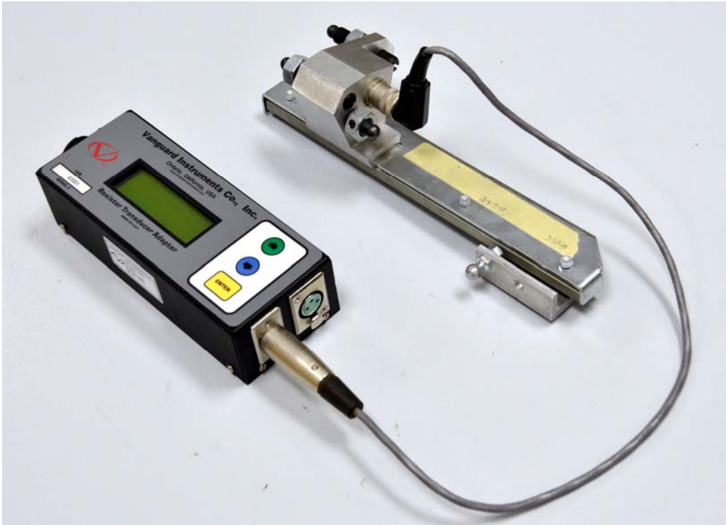
Figure 1. Typical Connection to ABB AHMB Transducer
